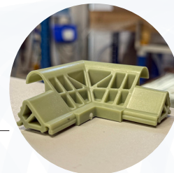
We use it for producing corners for FBS panels.
